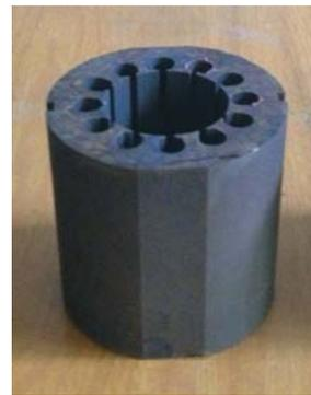
(b)非晶层间无绝缘黏结剂的定子铁芯
