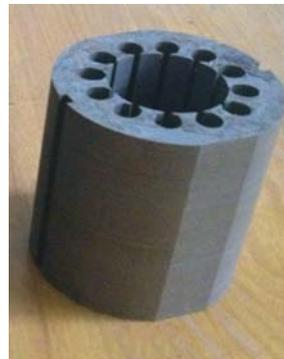
(c)非晶层间有绝缘黏结剂的定子铁芯
