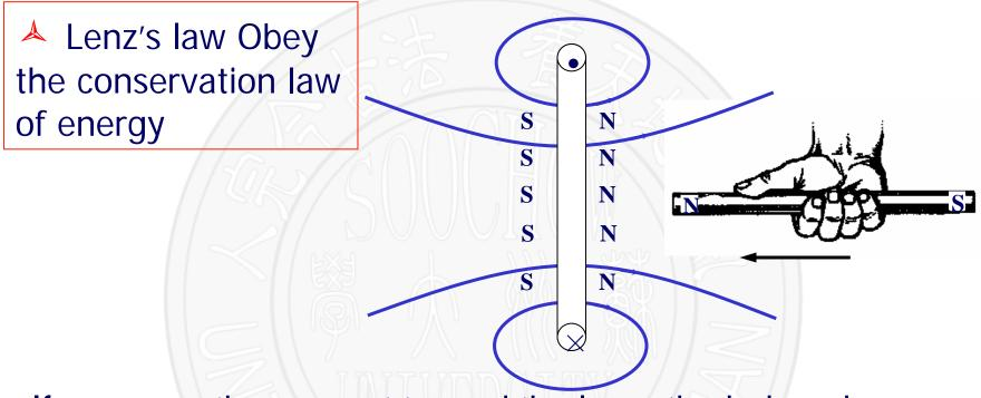
If we move the magnet toward the loop, the induced current points as shown, setting up a magnetic field that oppose the motion of the magnet.
