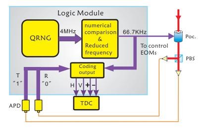
Fig. 2. A Logic Module is applied for controlling the Pockels Cells, switching polarization bases and outputting measurement results. Commercial QRNGs are applied to choosing measurement basis. The logical operation and the human-computer interface are realized via a CPLD (Complex programmable logic device) chip and a Single-Chip Microcomputer.
