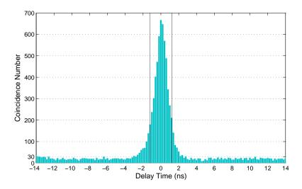
Fig. 3. The coincident detection events between Alice and Bob in a 25-min continuous sampling test. After balancing the number of coincident events and the source visibility, we set the gate width to be 2.5 ns in our experiment.
