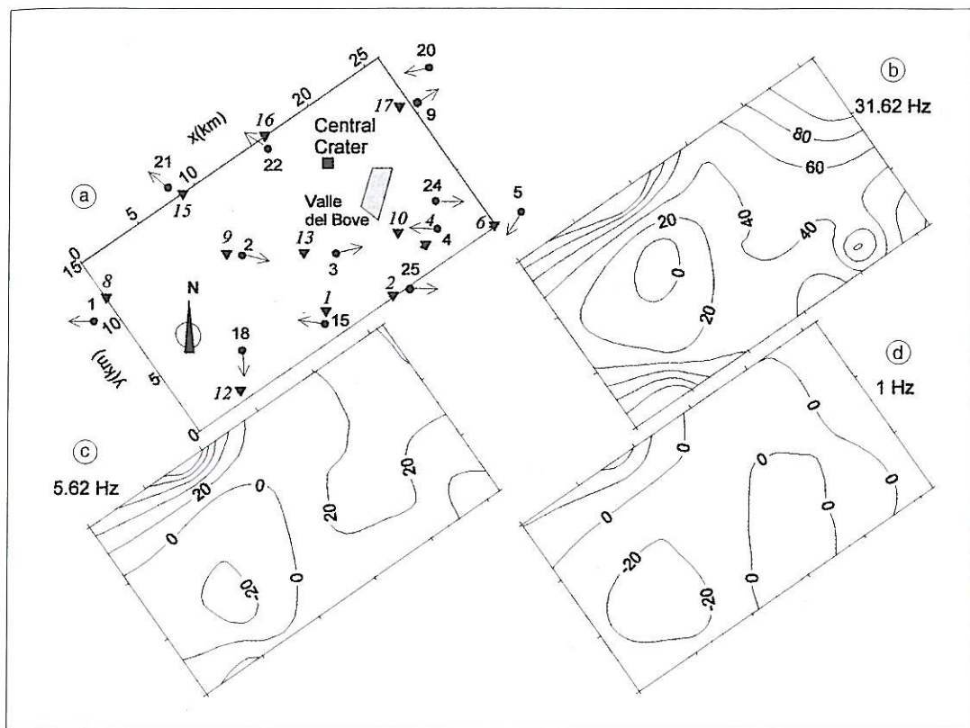
Fig. 6a-d. The Percent Discrepancy Parameter (PDP) representation. a) The MT and DES stations location map; b,c,d) the PDP horizontal frequency slices.
