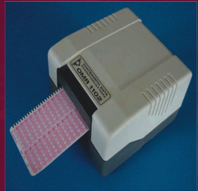
FIGURE 4-13 Optical mark readers. OMR readers are commonly used to score tests and tally questionnaires.
