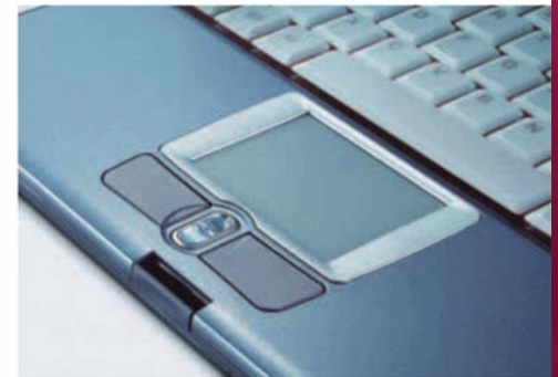
TOUCH PAD Commonly found on notebook PCs, keyboards, or as a stand-alone device.
