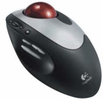
TRACKBALL Takes up less desk space than a mouse and is easier for some users to manipulate.
