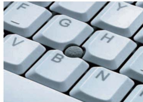
POINTING STICK Found on some notebook PCs. The stick is pushed in different directions to move the onscreen pointer.
