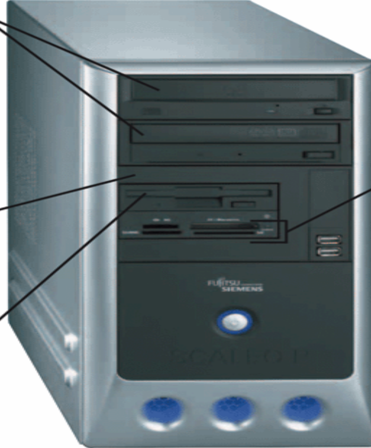
FIGURE 3-1 Storage device identifiers. To keep track of storage devices in an unambiguous way, the computer system assigns letters of the alphabet or names to each of them.
