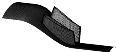
图4 原始造型过渡段计算区域及表面网格示意图 Fig. 4 Schematic diagram of calculate domain and surface mesh of original geometric modeling gooseneck
