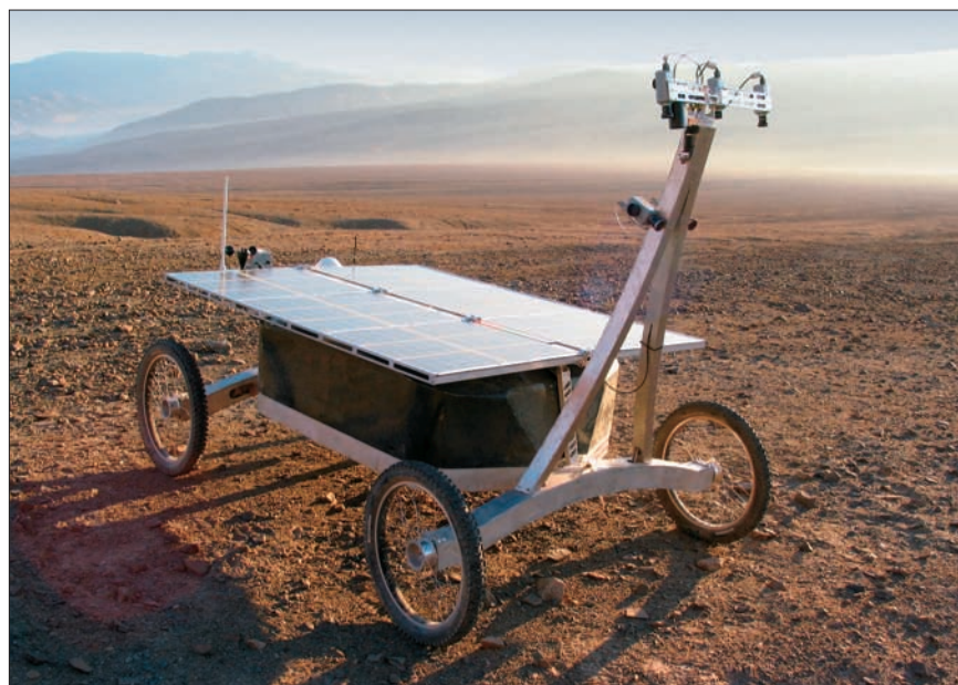
Figure 1. Zoë, the “robotic astrobiologist” created for the Life in the Atacama project.
