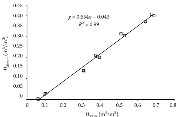
Figure 5. Laboratory calibration curve obtained in a box with quartz sand and its linear regression line (1)
