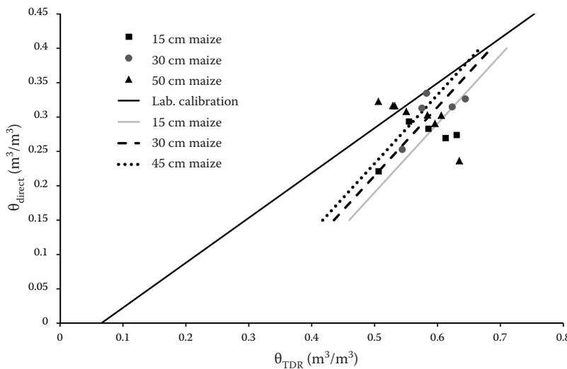
Figure 4. Field calibration of three Aqua-Tel-TDR sensors under maize between 8 March and 22 October 2010; the groups of points for individual sensors are approximated by Eq. (2); the laboratory calibration curve (Eq. (1) and Figure 5) is plotted for comparison
