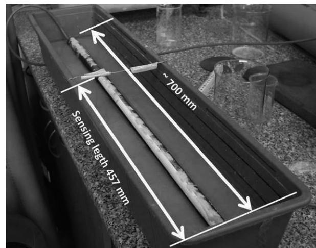
Figure 1. Overall appearance of the Aqua-Tel-TDR sensor during laboratory calibration
