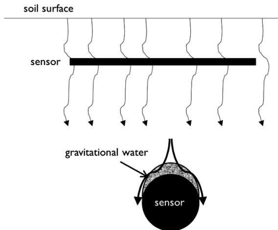
Figure 2. Schematic diagram of probable mechanisms of the preferential flow sensing by the Aqua-Tel-TDR sensor
