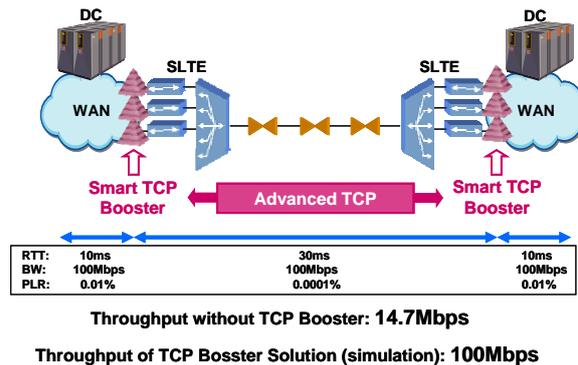
Fig.6: Smart TCP Booster concept for latency unaware TCP transmission and its performance simulation example.
