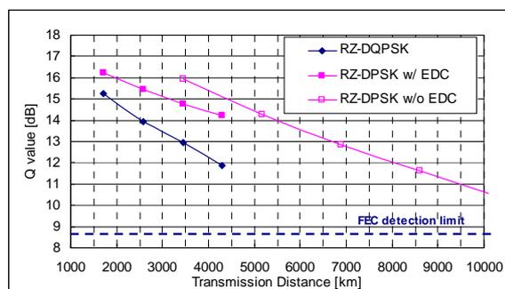
Fig.7: Q values v.s. transmission distance for 40 Gb/s x 32 DWDM, RZ-DPSK and 40Gb/s x 64DWDM RZ-DQPSK transmissions.
