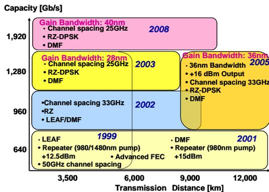
Fig.1: 10 Gb/s DWDM technology development in NEC for submarine cable systems.
