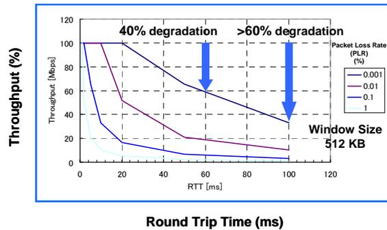
Fig.5: An example of TCP performance degradation by round trip time or line latency.
