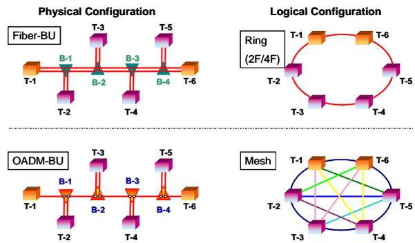
Fig.3: Comparison of physical and logical configurations between non-OADM and OADM systems.
