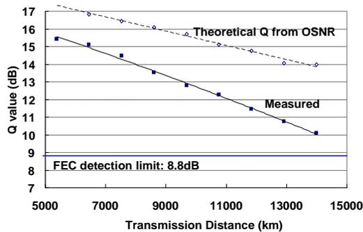
Fig.2: Q values v.s. transmission distance for 10Gb/s x 132 DWDM transmission.
