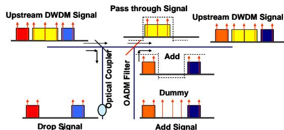
Fig.4: Optical add/drop branching architecture.
