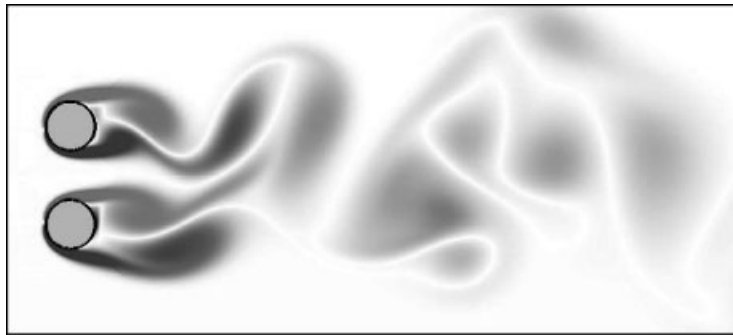
Figure 2. Contour plot of vorticity of an in-phase vortex street past a circular cylinder pair, Re_d = 150 , g = 1 .
