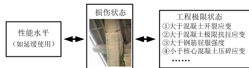
图 8 性能水平、损伤状态和工程极限状态关系 Fig.8 Relationship between performance level, damage state, and engineering limit state
