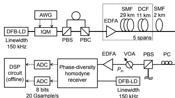
**Fig. 1:** Experimental setup for transmission of the 100-Gbit/s 32-QAM dual-polarization signal.
