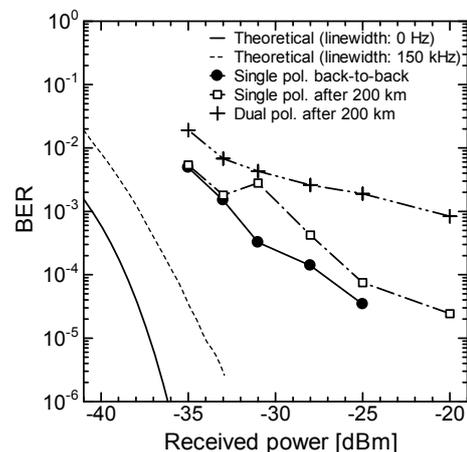
**Fig. 3:** BER characteristics of 32-QAM signals measured as a function of the received average power.
