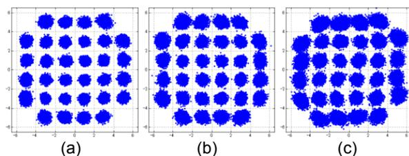
**Fig. 2:** Examples of constellation maps of 32-QAM signals when  $P_{in} = -20$  dBm, (a) single-polarization back-to-back, (b) single-polarization after 200-km transmission, and (c) dual-polarization after 200-km transmission.
