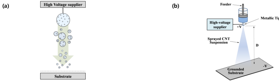
Fig. 1. Schematic explanation of (a) the operation principle, and (b) the experimental setup of the electro spray scheme. In (b), the spray angle is 30, and D is the nozzle-substrate distance.
