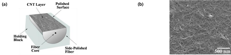
Fig. 2. (a) Prepared side-polished fiber deposited with CNTs onto a flat surface resulting in evanescent field interaction of the traveling mode with CNTs. (b) SEM image to evaluate the nano-morphology of the electro-sprayed CNT layer.
