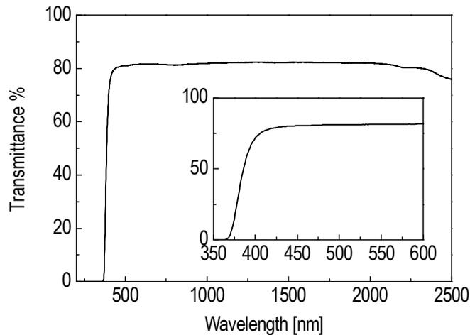
Fig. 2. Transmittance spectrum of BBT361. The sample thickness is 2 mm.
