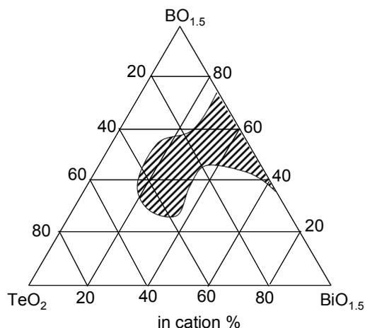
Fig. 1. Glass forming region (shaded area) of BTB glass system plotted in cation %, In  $\text{TeO}_2 > 60\%$ , no investigation was done in this work.
