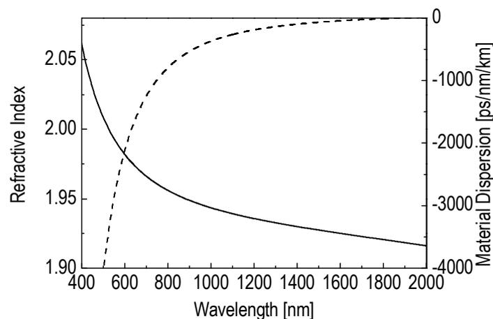
Fig. 3. Wavelength dependence of refractive index (solid line) and material dispersion (dashed line) of BBT361.
