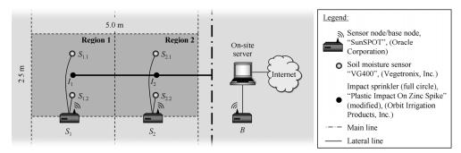
Figure 1. Schematic of the soil moisture monitoring system
