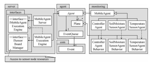
Figure 2. Abridged UML class diagram detailing relevant classes embedded in the wireless sensor nodes
