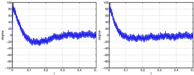
Fig. 7. Phase error of Simulink simulation. Left: linear design. Right: nonlinear design.
