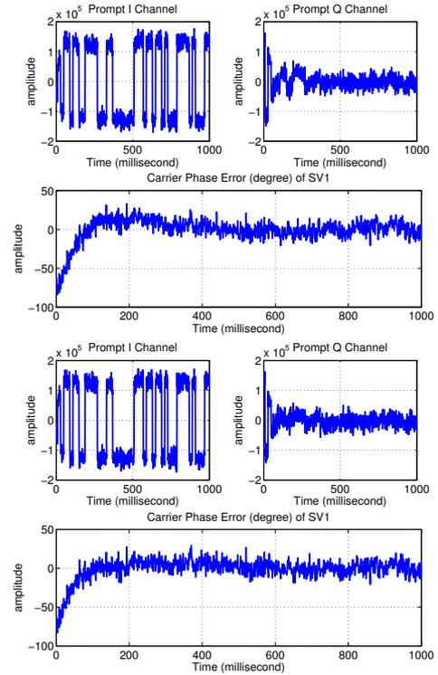
Fig. 8. Real GPS experimental results. Up: linear design. Down: nonlinear design.
