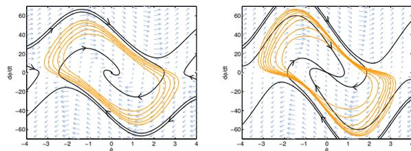
Fig. 6. Comparison of the domain-of-attraction. Left: linear design. Right: nonlinear design.
