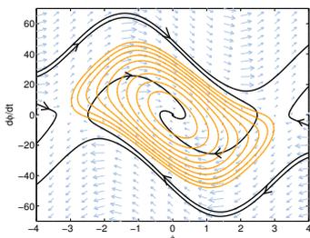
Fig. 5. Local Lyapunov level sets of the original PLL system.
