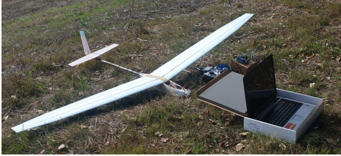
Figure 6 The UAV system, including the ground station.
