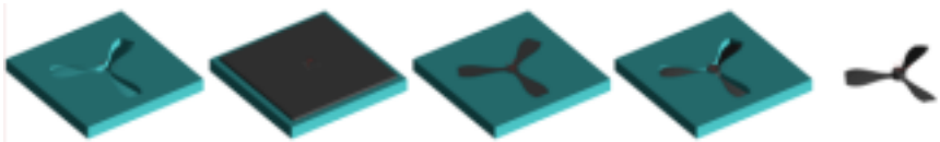
Figure 9. Steps in rotor fabrication
