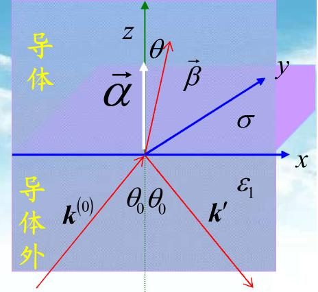
$$\boxed{\begin{aligned} \beta_z^2 &= \frac{1}{2}(\omega^2 \mu \varepsilon - \beta_x^2) + \frac{1}{2}[(\omega^2 \mu \varepsilon - \beta_x^2)^2 + \omega^2 \mu^2 \varepsilon^2]^{1/2} \\ \alpha^2 &= -\frac{1}{2}(\omega^2 \mu \varepsilon - \beta_x^2) + \frac{1}{2}[(\omega^2 \mu \varepsilon - \beta_x^2)^2 + \omega^2 \mu^2 \varepsilon^2]^{1/2} \end{aligned}}$$
