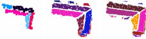
Figure 4. Left: planar segments detected in the DSM (fig. 3). Centre/right: Homogeneous segments from two aerial images projected to the DSM. Resolution: 0.1 m.
