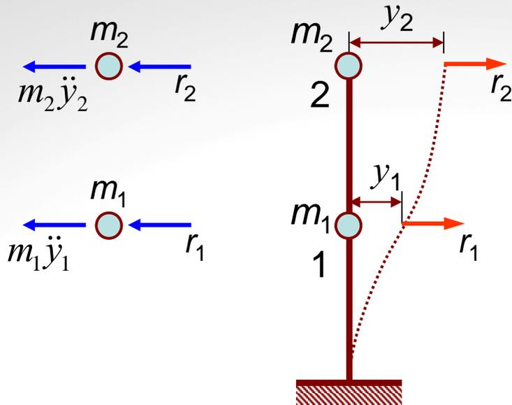
$$\left. \begin{aligned} m_1\ddot{y}_1 + r_1 &= 0 \\ m_2\ddot{y}_2 + r_2 &= 0 \end{aligned} \right\}$$
