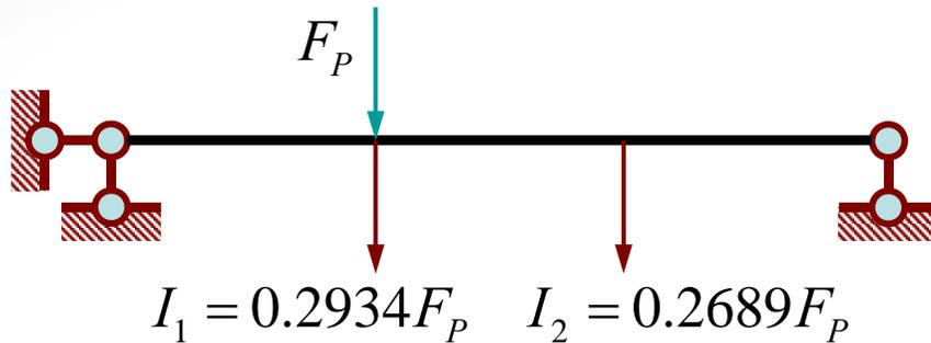
$$M(t)_{\max} = \bar{M}_1 I_1 + \bar{M}_2 I_2 + M_P$$
