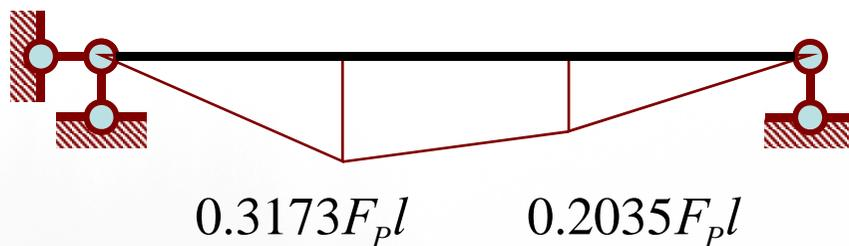
$$M_{1\max} = \bar{M}_{11} I_1 + \bar{M}_{12} I_2 + M_{1P}$$
