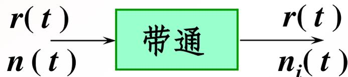
$$r(t) + n_i(t) = \begin{cases} a \cos \omega_c t + n_i(t) & \text{发“1”} \\ n_i(t) & \text{发“0”} \end{cases}$$
