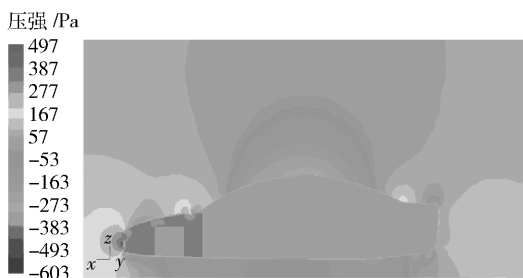
图 7 车速 100 km/h 时 y=0 m 截面的压力场分布 Fig. 7 Pressure field distribution of vehicle at 100 km/h for y=0 m
