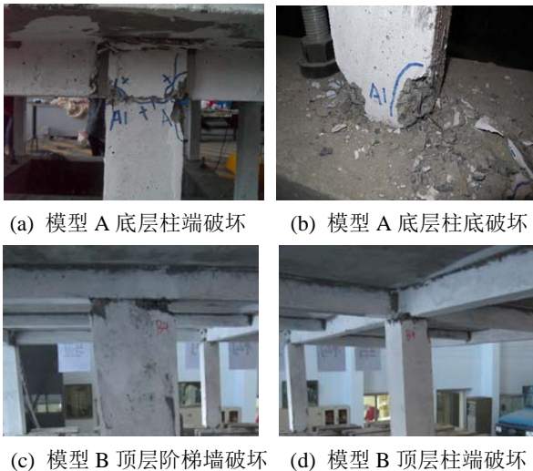
图 10 T6 极震工况下模型破坏情况 ( A_{max}=0.91g ) Fig.10 Damage observed during T6 ( A_{max}=0.91g )
