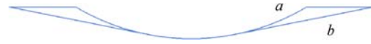
图7 纤维束轨迹挤压变形和打紧示意图 Fig. 7 Sketch of extrusion deformation and jamming of fiber bundle trajectory
