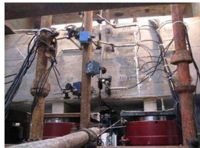
图 11 管片接头抗弯试验加载实况 Fig.11 The bending test of segmental joint
