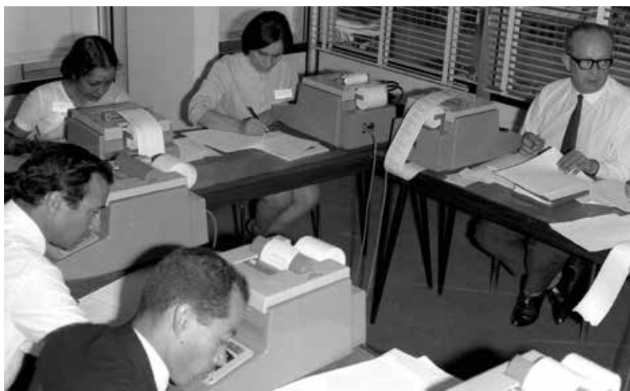
Students at work with mechanical calculating machines, the tools usually available in the late 1960s for statistical analyses of epidemiological data sets. Beyond the four arithmetic operations, these machines could calculate the sum of a sequence and the sum of the products of two sequences of numbers.
