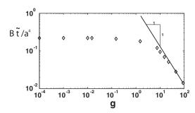
FIG. 2. The scaled step collapse time  $\tilde{t}$ ,  $\tilde{t} = t_n/n^4$  for  $n \gg 1$ , as a function of the relative step interaction strength, g, for an initial cone of unit slope; B is a material parameter. Symbols are step simulation data and the solid line is our prediction,  $\tilde{t} = O(g^{-1})$  for  $g \gg 1$ .
