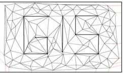
(b) Delete "R" and insert "GI" as constraint edge
