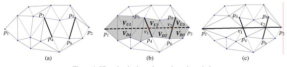
Figure 1. Virtual point insertion and re-triangulation. (a) original CD-TIN before inserting constrained edge  $p_1p_2$ . (b) Influence domain of  $p_1p_2$  and the intersect point
