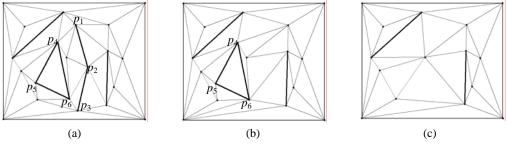
Figure 5. To delete constraint edges without virtual point
