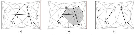
Figure 6. To delete constraint edges with virtual point
