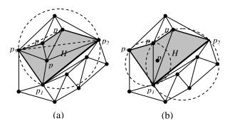
Figure 3. Deletion of non-constraint point p
