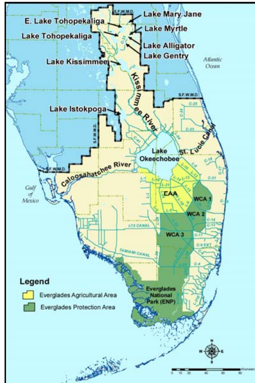
Figure 2. The South Florida Water Management District with water management infrastructure (canals, lakes and impoundments).
