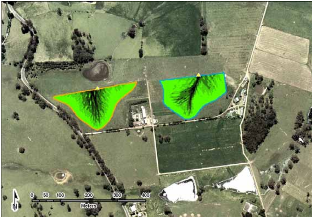
Figure 3. Spatial distribution of ATB for dryland catchments. Low (light green) – high (dark green).
