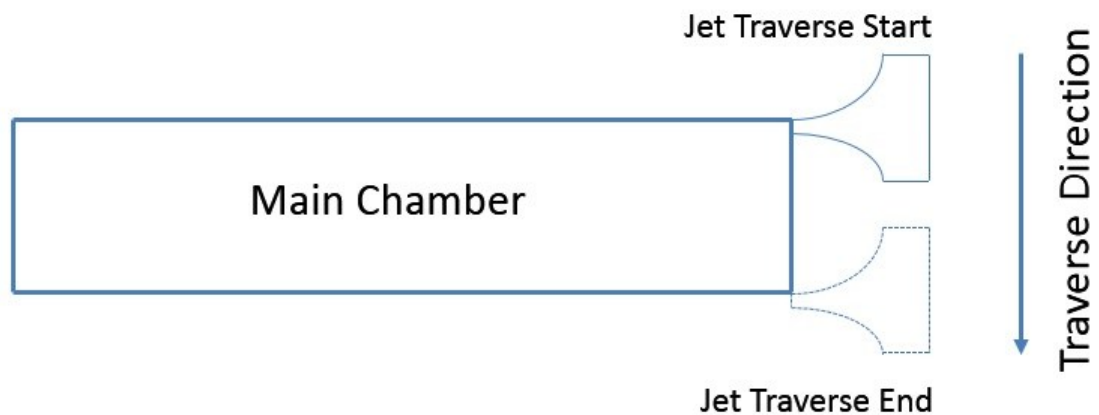
Figure 4. 7 Schematic illustrating the position of the nozzle at the start of jet traverse and at the end.
