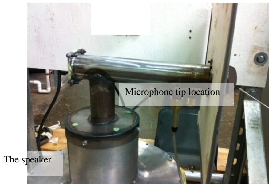
Figure 4.9 The 10 inch speaker resonance test apparatus
