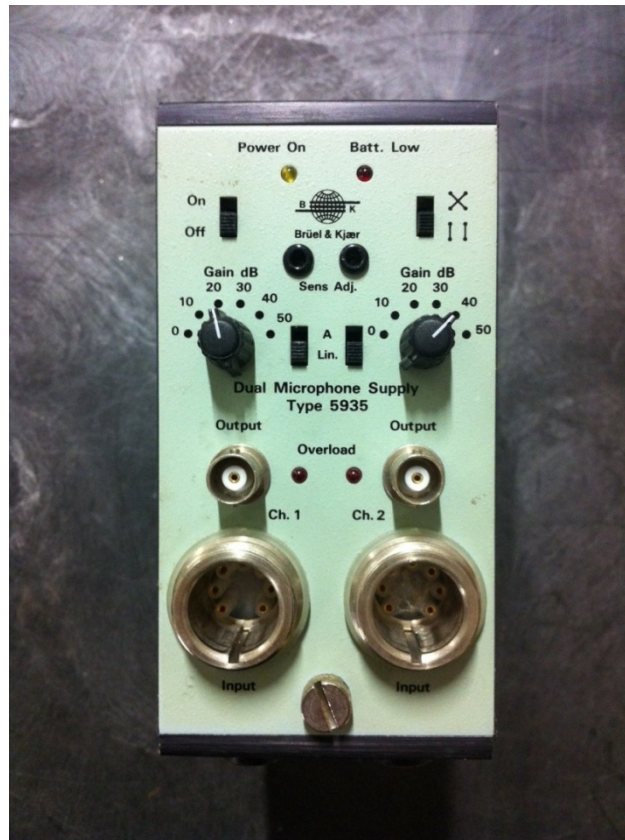
Figure 3.12 The dual microphone supply and preamplifier
