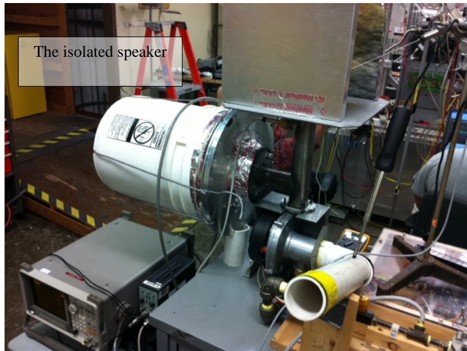
Figure 4.21 Apparatus with the 10 inch speaker, bucket isolation
