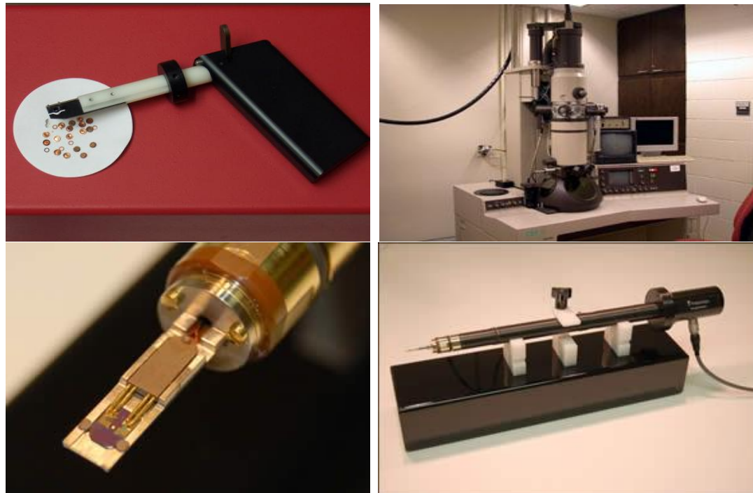
Figure 2.4 Cryo-TEM ultra-rapid sample freezing system
