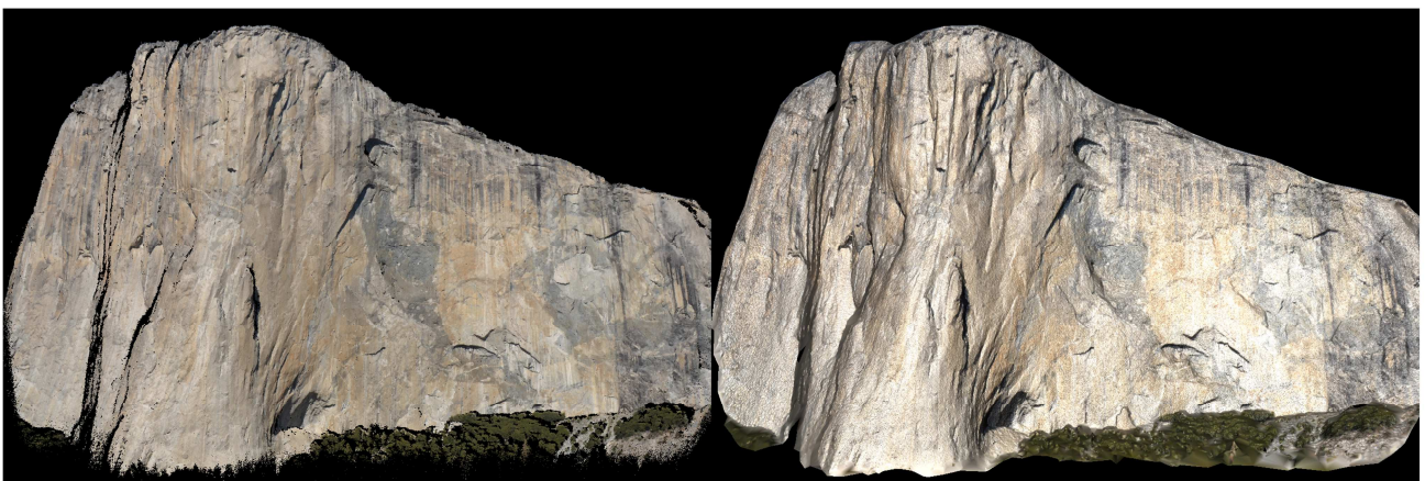
Fig. 3.4: Left: resulting point cloud after stereo models selection and dense image matching with SURE . Right: triangle mesh derived from point cloud. Point cloud count original: 146 Mio. pts. Filtering with maximum occurrence 1: 31 Mio. pts., mo 2: 18 Mio. pts., mo 4: 11 Mio. pts.
