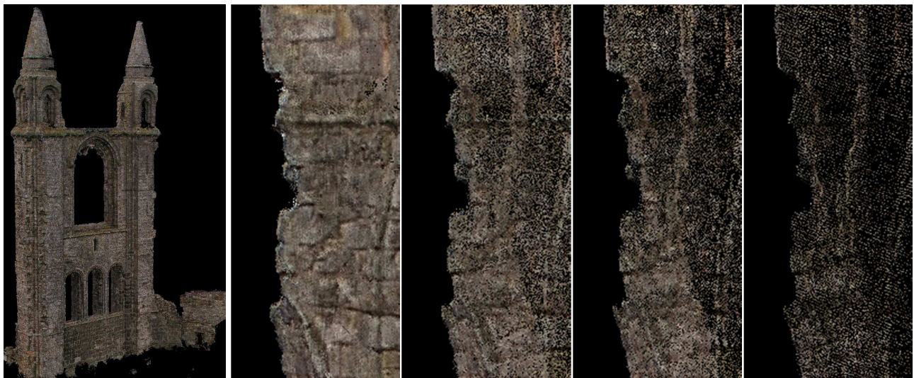
Fig. 2.4: Resulting point cloud after stereo models selection and dense image matching with SURE . Left: full view, filtered with maximum occurrence 1. Right: Detail from full cloud (49.1 Mio. pts.), filtered with mo 1 (7.1 Mio. pts.), filtered with mo 2 (3.8 Mio. pts.), filtered with mo 4 (1.9 Mio. pts.)
