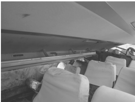
图6 实际事故中大客车生存空间压缩图 Fig. 6 Residual space intruded in real accident
