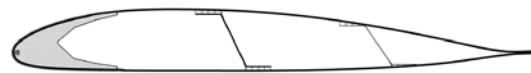
图 5 “海豚”直升机桨叶 0.4R 处的参数化剖面 Fig. 5 Parametrization model of the “Dolphin” helicopter’s blade 0.4R section
