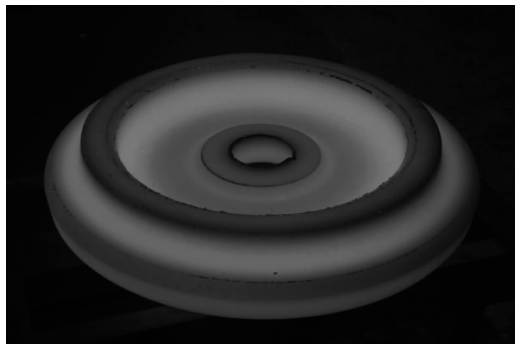
图2 某型发动机用TA29钛合金整体叶盘锻件 Fig.2 TA29 titanium alloy blisk forging for an advanced aeroengine
