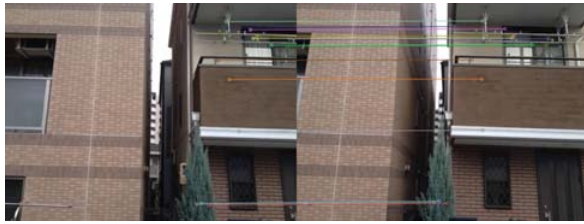
Figure 5. Correction of matching results by RANSAC
