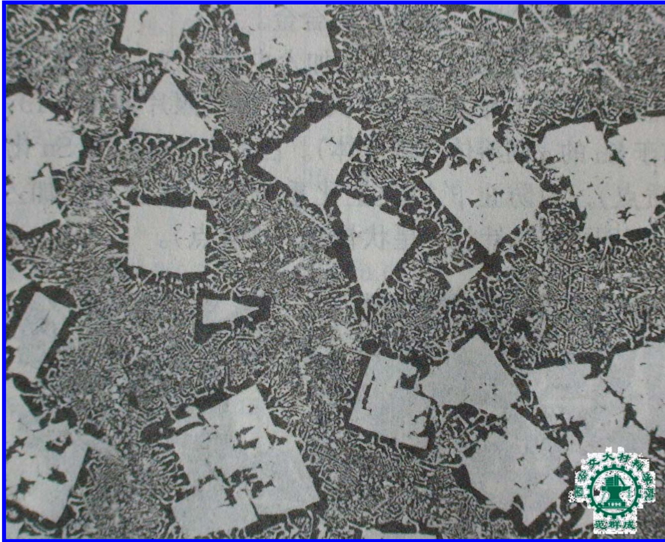
The microstructure of ZPbSb16Sn16Cu2 sliding bearing alloy
