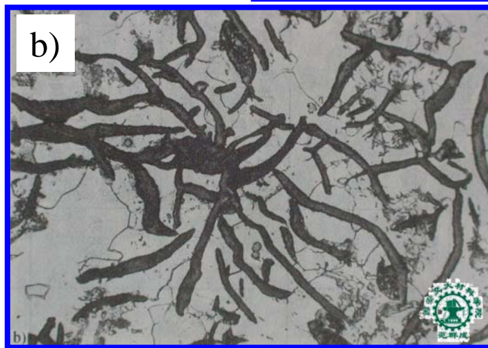
Structures of common gray cast iron a) F+G 片 b) F+P+G 片 c) P+G 片
