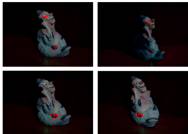
Figure 6: Matched points on pairs formed by the right image of the first scan position (left) with the left image (above) and the right image (below) of the second scan position.
