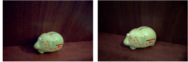
Figure 3: Matched points on the right image from the first scan position and the left image from the second scan position.
