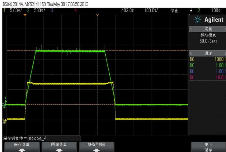
Figure 9. Power supply normal output voltage and current waveform
