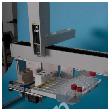
图 1 OPTIC 2 多模式进样口及 CONCEPT 多功能前处理装置 Fig. 1 The OPTIC 2 system of multi-modal injector and CONCEPT multi-functional preparation sample pre-treatment device
