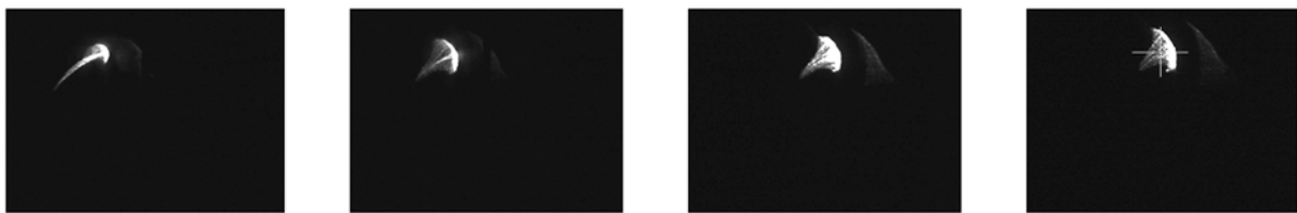
(a)最初焦斑图像 (b)水平调节时的焦斑图像 (c)轴向调节时的焦点图像 (d)调节结束时的焦点图像 (a) Initial focus image (b) Focus image during level adjustment (c) Focus image during axial adjustment (d) Focus image at end of adjustment
