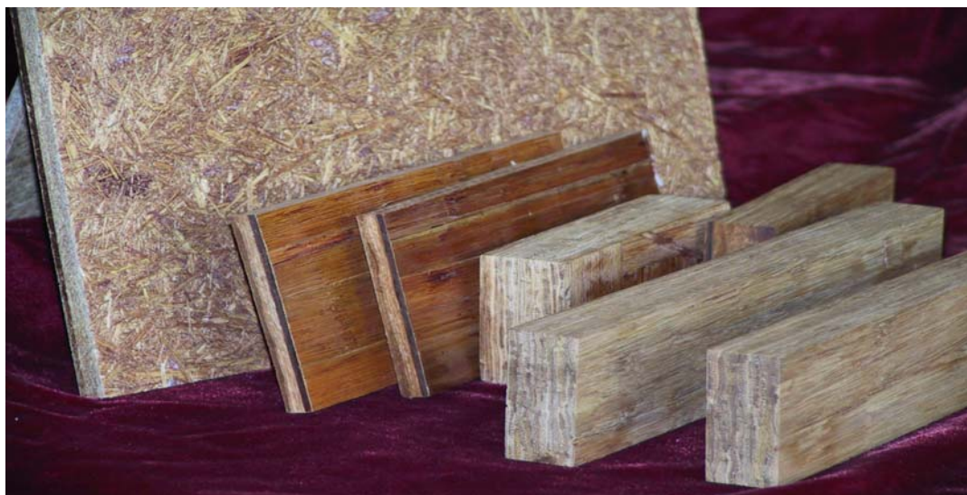
Fig. 1 the panels laminated along the grain and cross grain, as well as the bamboo flake board for architecture wall material
