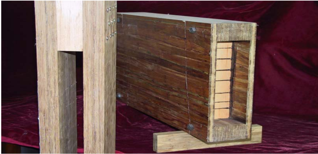
fig.2. The samples of the molding structure component, box-beam and splint-column made from bamboo laminated panels
