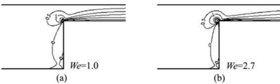
图 7 收缩口附近 T_{xy}^1 等值线 Fig. 7 The T_{xy}^1 contours near to sharp corner
