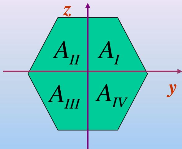
$$\begin{aligned}\int_{A_I} yz dA &= -\int_{A_{II}} yz dA \\ &= \int_{A_{III}} yz dA = -\int_{A_{IV}} yz dA\end{aligned}$$
