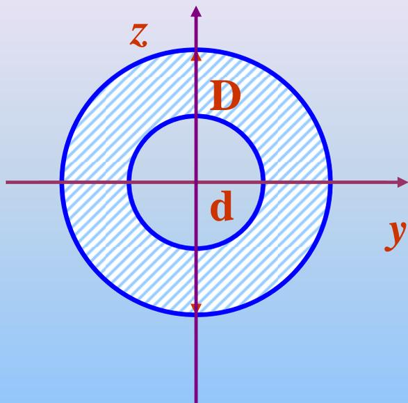
$$\begin{aligned} I_P &= I_{P\text{大}} - I_{P\text{小}} \\ &= \frac{1}{32} \pi D^4 - \frac{1}{32} \pi d^4 \\ &= \frac{1}{32} \pi D^4 (1 - \alpha^4) \end{aligned}$$
