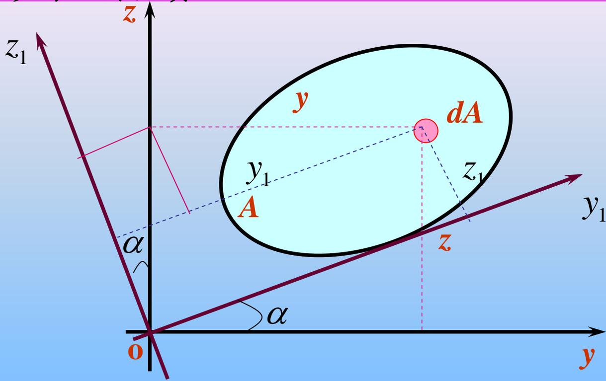
$$\begin{aligned} I_{y_1 z_1} &= \int_A y_1 z_1 dA = \int_A (y \cos \alpha + z \sin \alpha)(z \cos \alpha - y \sin \alpha) dA \\ &= \int_A (z^2 - y^2) \sin \alpha \cos \alpha dA + (\cos^2 \alpha - \sin^2 \alpha) \int_A yz dA \end{aligned}$$
