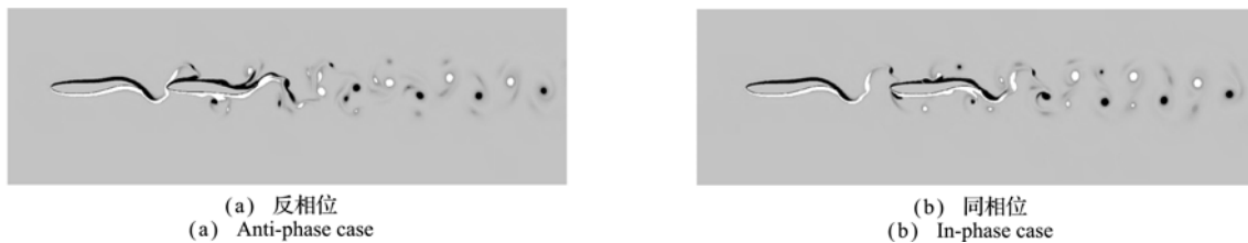
图 7 t/T=20.50 时的涡量图 ( d_0=0.5 ) Fig. 7 Vorticity field around two fish at t/T=20.50 ( d_0=0.5 )
